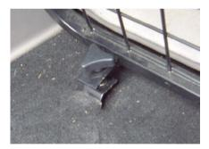
Now position the Dog Guard so that the slotted bracket fits around the rear seat catch. See photograph 3. When the seats are up right they hold the guard in position.
